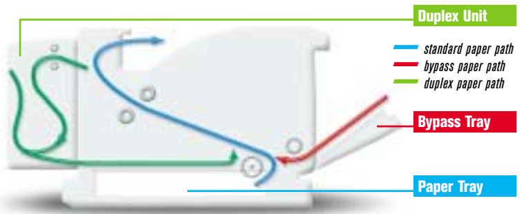
A short paper path provides higher throughput and reliability.
